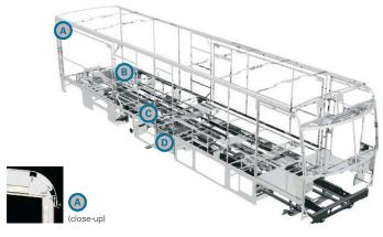
**SUPERSTRUCTURE** is the term given to Winnebago Industries' structural motor home design and construction. Rather than a single component, it is the culmination of design integration that incorporates steel and aluminum substructures; composite-design laminated floor risers; interlocking joint technology; and Thermo-Panel® floor, roof and sidewalls to form a high-strength, durable vehicle body.
