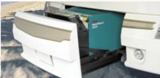
Main: QS40C • Charleston Below: 8.0 kW diesel generator on slide-out caddy
