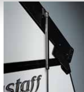
Gas Strut Lift Assist (Std. Hard Side Models w/ Manual Lift Roof Only)
