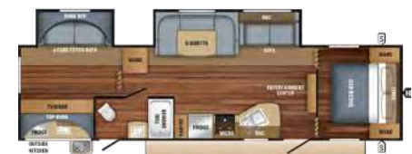
JAY FLIGHT SLX | 324BDS OPTION A Ext. Lgth: 36' 2" Ext. Ht: 134" Unloaded Wt. (lbs): 7,615 Sleeps: 6-10
