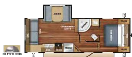
JAY FLIGHT SLX | 245RLS OPTION A Ext. Lgth: 28' 2" Ext. Ht: 132" Unloaded Wt. (lbs): 5,220 Sleeps: 4-6
