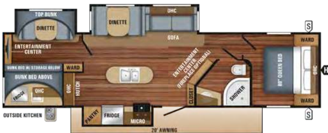
JAY FLIGHT | 33RBTS OPTION D Ext. Lgth: 37' 8" Ext. Ht: 134" Unloaded Wt. (lbs): 8,600 Sleeps: 7-9
