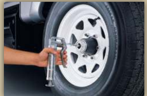
Jay Flight's E-Z Lube® axles with removable caps make maintenance a snap.
